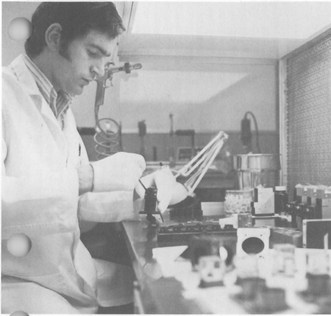
In Q.A. metrology area, Ed Knezivech uses interferometer technique to determine flatness of surface of cube corner. Every optics product is similarly checked prior to final assembly and shipment.
